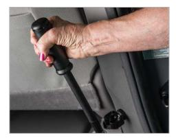
**Easy Manual In-Floor Ramp** Easy to use for caregivers of any age or size, requiring no bending or heavy lifting.
